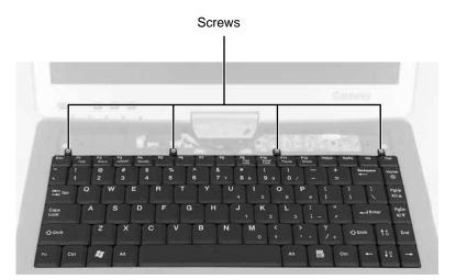
14 Lift the back edge of the keyboard, then slowly rotate it toward you so it lies **keys-down** on top of your convertible tablet PC. Be careful not to damage the LCD panel or unplug the keyboard ribbon cable.
